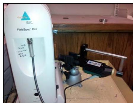
FIG. 2 PLANT PROBE AND ASD FIELD SPEC PRO HR SPECTROMETER
